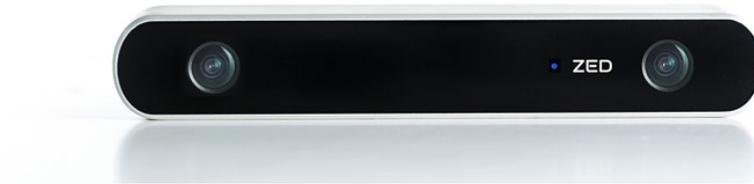
Fig. 24. The ZED depth camera. Image credit: Stereolabs
